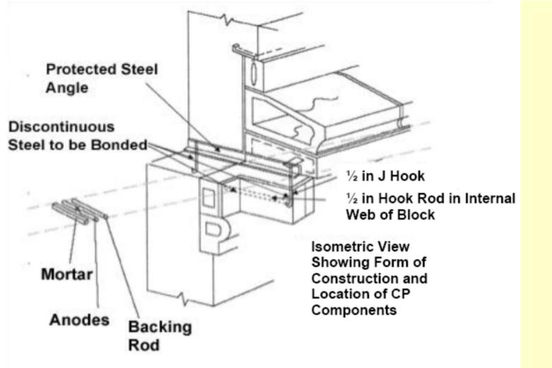
Failure to bond the discontinuous metal may result in either (i) cracking of the terra cotta modillion unit, or (ii) accelerated corrosion of the J hook support and potential spalling to ground level.
